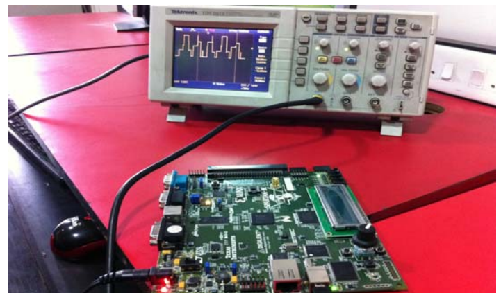
Fig 5. Output of VHDL code burnt on kit for DAC interfacing tested on DSO.
